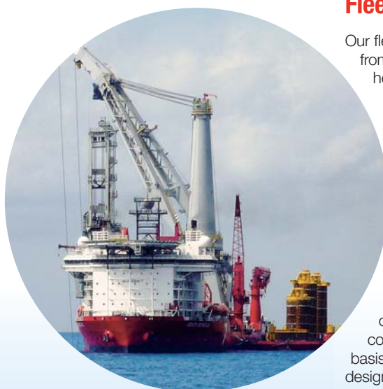
Seven Borealis operating in J-lay mode offshore Angola
